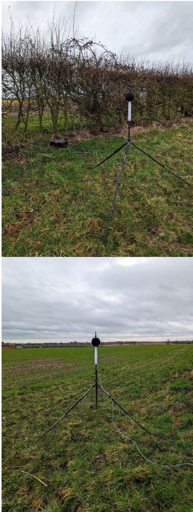
Figure 2: Photographs of baseline noise monitoring equipment at Location B
