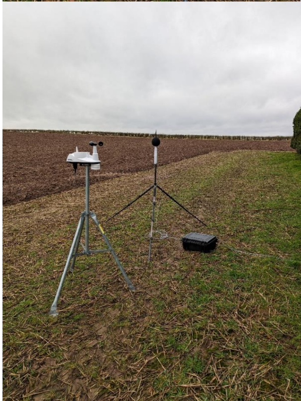
Figure 3: Photographs of baseline noise monitoring equipment at Location C
